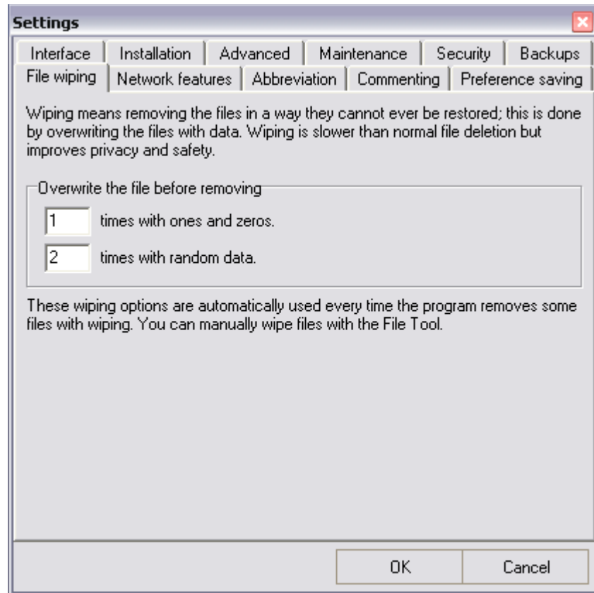
Image 9. You can adjust the strength of the file wiping to meet your requirements
